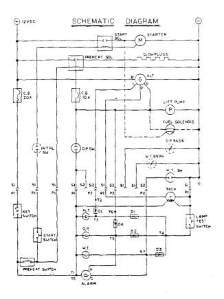
START : I. TURN KEY TO ON POSITION. THE ALARM WILL SOUND, OIL PRESSURE AND BATTERY CHARGE INDICATORS WILL LIGHT.
