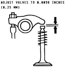
Adjusting a valve's clearance with a feeler gauge.
