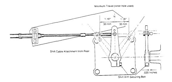
NOTE: Excessive throw distance in the remote control lever is not detrimental to the transmission. Note that the position of the remote control lever should align with the NEUTRAL marking on its bracket when the transmission is really in NEUTRAL.
