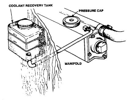
Coolant Recovery Tank, Recommended Installation
