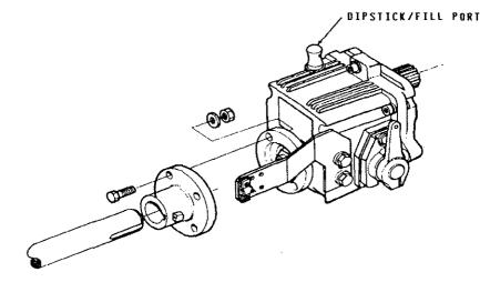
Change the transmission oil after the first 30 hours of engine operation and thereafter every 250 hours (or once per year, minimum). The BW 3 transmission has a drain plug for draining the old transmission fluid. To ensure that most of the old oil is drained from the transmission, run the engine in NEUTRAL for approximately 10 to 15 minutes so the transmission oil may warm and flow better from the transmission. This
