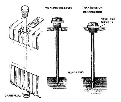
The Transmission drain plug is located directly below the dipstick and is the same size hex head as the dipstick. This drain plug also has a sealing washer.
