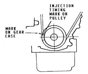
If the specified injection timing (25° BTDC) cannot be attained, adjust the timing by increasing or decreasing the thickness of the injection pump mounting shim. Changing the shim thickness by 0.004 inch (0.01mm) changes the injection timing by approximately one degree. To advance the timing, decrease the shim thickness, as required. To retard the timing, increase the shim thickness, as required. Refer to your engine's parts List for shim part numbers.
