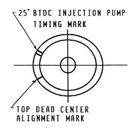
3. Facing the front of the engine, rotate the crankshaft 170° clockwise to position the No. 2 piston at TDC of its compression stroke. Now adjust the No. 2 piston's intake and exhaust valves.
