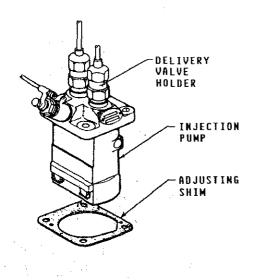
Fuel Injection Pump with an Adjusting Shim
