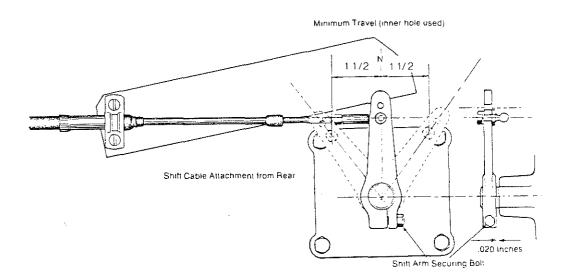
NOTE: If the throw distance (or travel) of the remote cable is too short, the gear box lever cannot fully engage the transmission into FORWARD or REVERSE. In this situation, the transmission's internal gears will wear prematurely and the transmission may over heat.
