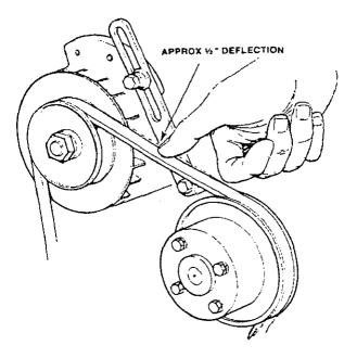
Alternator and Water Pump Belt Tension
