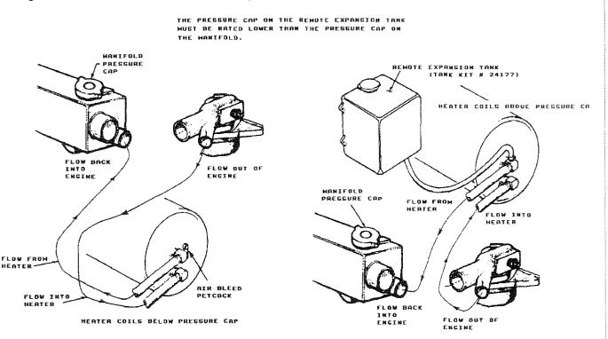
The illustrations shown above are Flow Control designs which have been adapted to operate with the single pass manifolds installed on the 12B TWO diesel engine.
