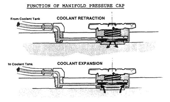
Coolant from the engine, when heated during engine operation, will expand, lifting the spring-loaded manifold pressure cap, and enter the recovery tank by way of the hose connecting the recovery tank to the manifold.
